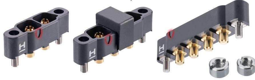
For the <u>male connectors</u>, these are also available in 2, 3 and 4-contact single row options for PCB throughboard mounting in vertical, with 4.5mm PC tails. They also display a contact no. 1 marker, and are supplied in tubes with pick and place caps fitted.
