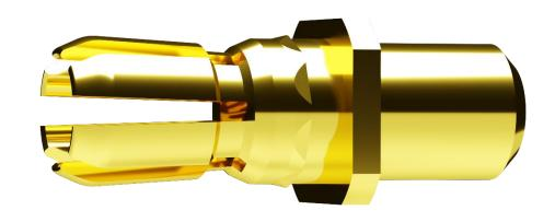
In contrast to the other <u>Hi-Rel connectors</u> (where the female contact is the heart), here you'll find a 6-fingered Beryllium Copper male contact providing a positive normal spring force against the female mating contact. The durable hard-acid gold finish ensures repeated mating cycles and long-term environmental exposure do not affect the connection surfaces.
