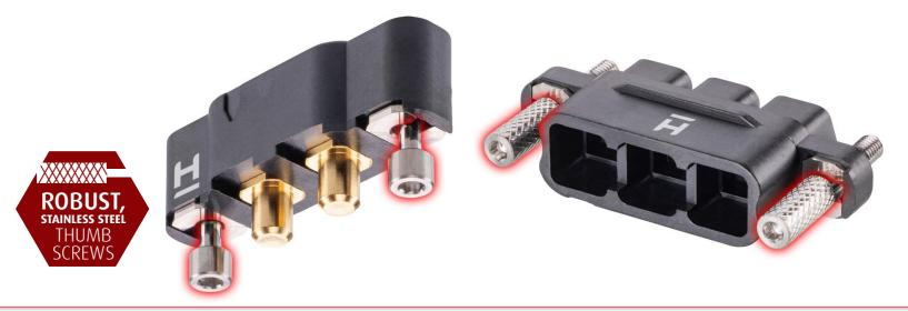
All Kona connectors are fitted with screw-lock fixings, to achieve the maximum vibration and shock specifications. They are also mate-before-lock, so connectors are easier and faster to mate before the screws are engaged and screwed together.
