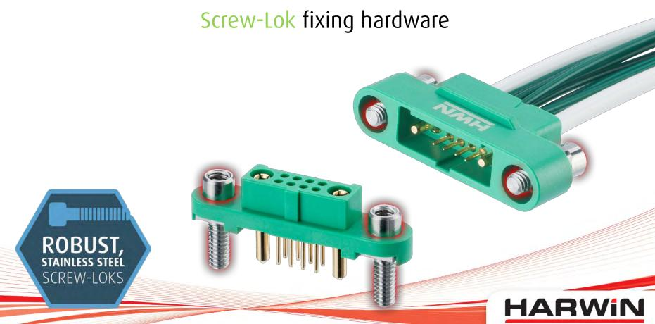
The captive screws with hex socket heads prevent slipping during assembly. The design of these captive screws allows for 'Mate before Lock' – connectors can be fully mated before the screws need to be engaged. This provides for faster and easier assembly.
